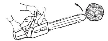
Improper thrust cutting.
